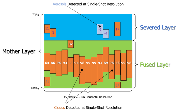
Figure 4: Schematic of a 5 km scene illustrating fused layer determination by identifying the maximum CAD score assigned to layers detected within each single shot profile. CAD scores for the features selected to define the upper boundary of the fused layer are shown in white.
