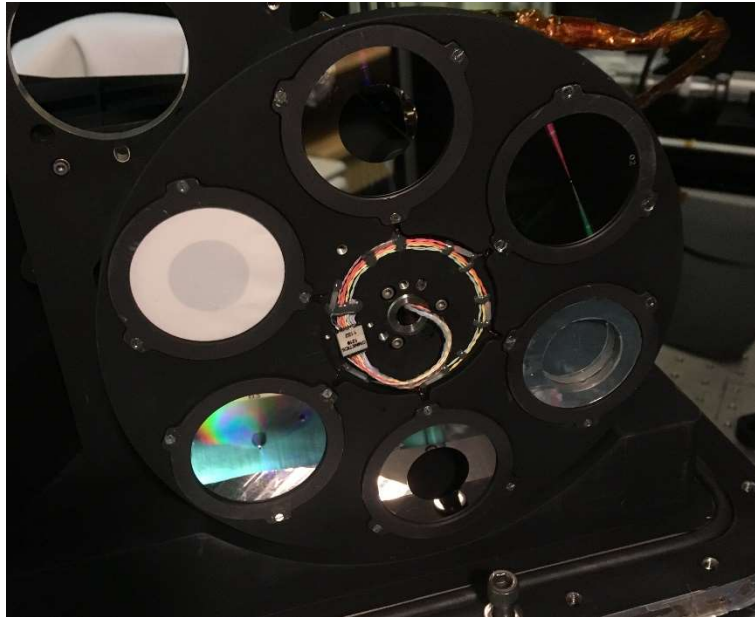
Figure 76. Transmissive diffuser mounted on the HySICS balloon instrument aperture wheel. The diffuser is a white piece of PTFE placed on top of an equivalent 20 mm aperture.
