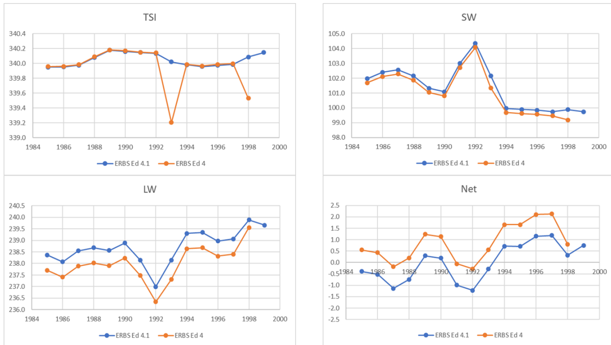
Figure 1. Comparisons between ERBS S10n Edition 4 (red) and Edition 4.1 (blue) time series of global annual mean TOA fluxes in Wm^{-2} from 1985 to 1999 for incoming solar radiation (TSI), reflected shortwave radiation (SW), outgoing longwave radiation (LW), and net downward radiation (Net).
