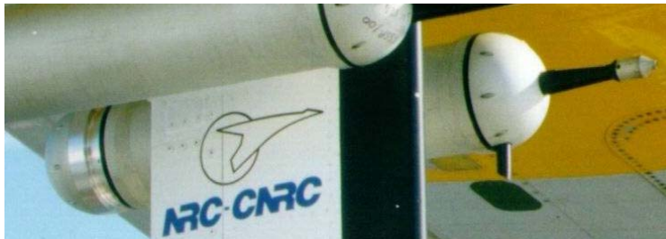
PCASP mounted on the NRC Convair 580 in FIRE ACE
