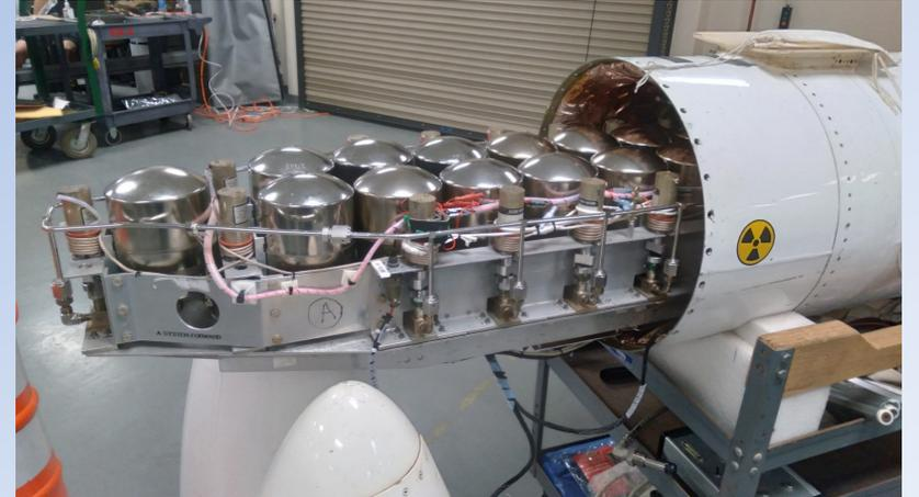
1. Manifold in ER-2 belly pod (nose cone off)
